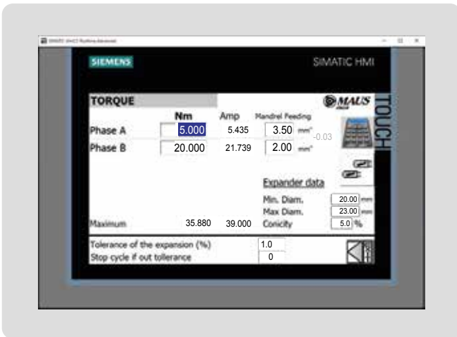
Torque values settings: Expansion torque phase "a" Mandrel feeding during phase "a" Expansion torque phase "b" Mandrel feeding during phase "b"
