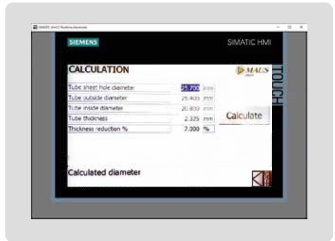
Digital calculation of nominal tube inside diameter after expansion considering the % of tube wall thickness reduction
