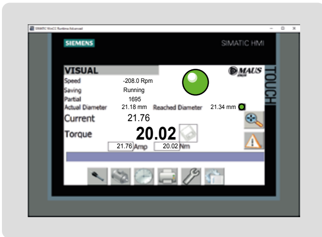
Expansion torque value in Nm Confirmation of reached the torque value Tube inside diameter reached after expansion in mm
