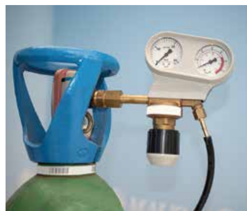
Pressure reducer for 50-litre argon cylinders
