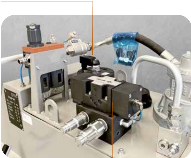
Pneumatic valves in manual / automated mode
