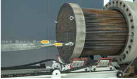
Pull the tubesheet with rope 2
